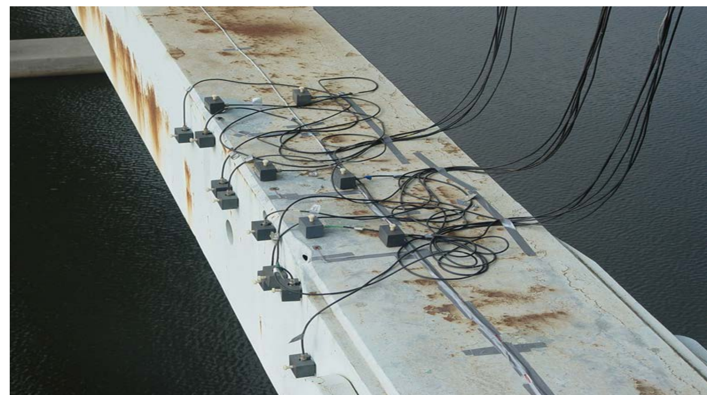
Figure 1. Acoustic Emission Monitoring of Concrete Girders (Courtesy Physical Acoustics Corp.)
