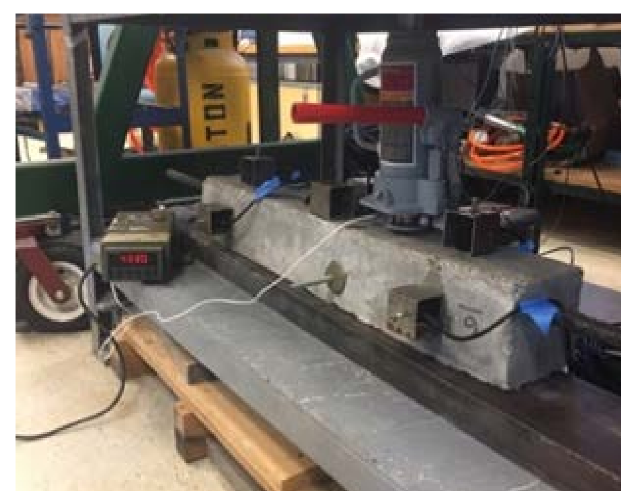
Figure 4. Sensor Array on Concrete Beam
